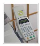
Thre COPICODE-IP improves the system of management and payment of printings to copiers not networked, via an alphanumerical identification code. By integrating the TCM2-MIFARE, it enables users' identification via a contactless MIFARE card or a 125 Khz.
